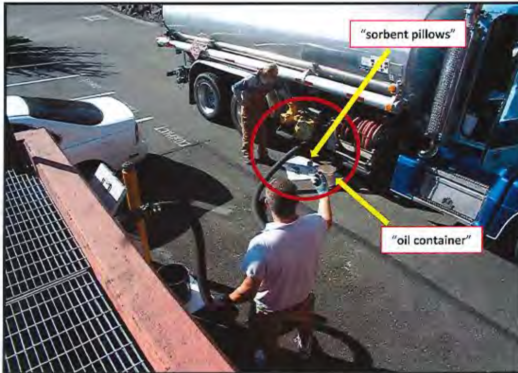
Figure 5: Correct way of loading and unloading diesel or gasoline using spill prevention and control equipment.
